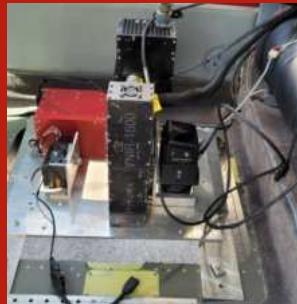
HSI camera systems built into a hatch
